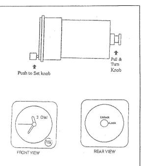
Caution! Do not push the setting Knob when the Locking knob is in the locked position. Pull the "Pull & turn knob" out all the way and then turn to the unlocked position.
